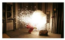
There are several ways to protect employees from arc flash such as work practices, insulation, guarding, barricades, and grounding. <u>PPE</u> is also available to protect against the possible injuries that can occur from an arc flash. Warning labels should be posted on equipment that is operating at 50 volts or more. The posting must also be
